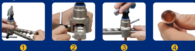
Usage method of quick-clamp
